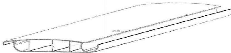
Fig. 12. LD01 slat model with a length of 4000 mm, adopted for the calculations.
