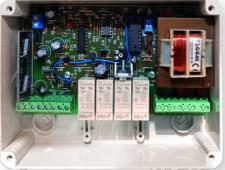
A photograph of the CRS-436XG control unit, similar to the CRS-435XG but with a more complex PCB layout, featuring two distinct channels and additional terminal blocks.                                  | Stk.    | 506,00 |
