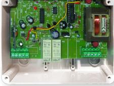
A photograph of the CRS-435XG control unit, showing a green printed circuit board (PCB) with various electronic components, including a red emergency stop button and a terminal block. | Stk.    | 394,00 |
