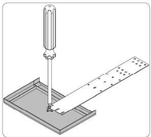
The screw is driven into the hole in the side cover using slight force.
